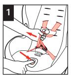
Loosen harness by pushing down on the harness release lever while pulling out on the harness. Undo harness retainer and unbuckle the buckle.
